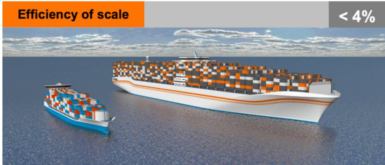
A larger ship will in most cases offer greater transport efficiency due to efficiency of scale. A larger ship can transport more cargo at the same speed with less power per cargo unit. Limitations may be met in port handling.
