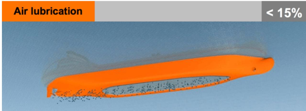
Compressed air is pumped into a recess in the bottom of the ship's hull. The air builds up a carpet that reduces the frictional resistance between the water and the hull surface. This reduces the propulsion power demand. The challenge is to ensure that the air stays below the hull and does not escape. Some pumping power is needed.
