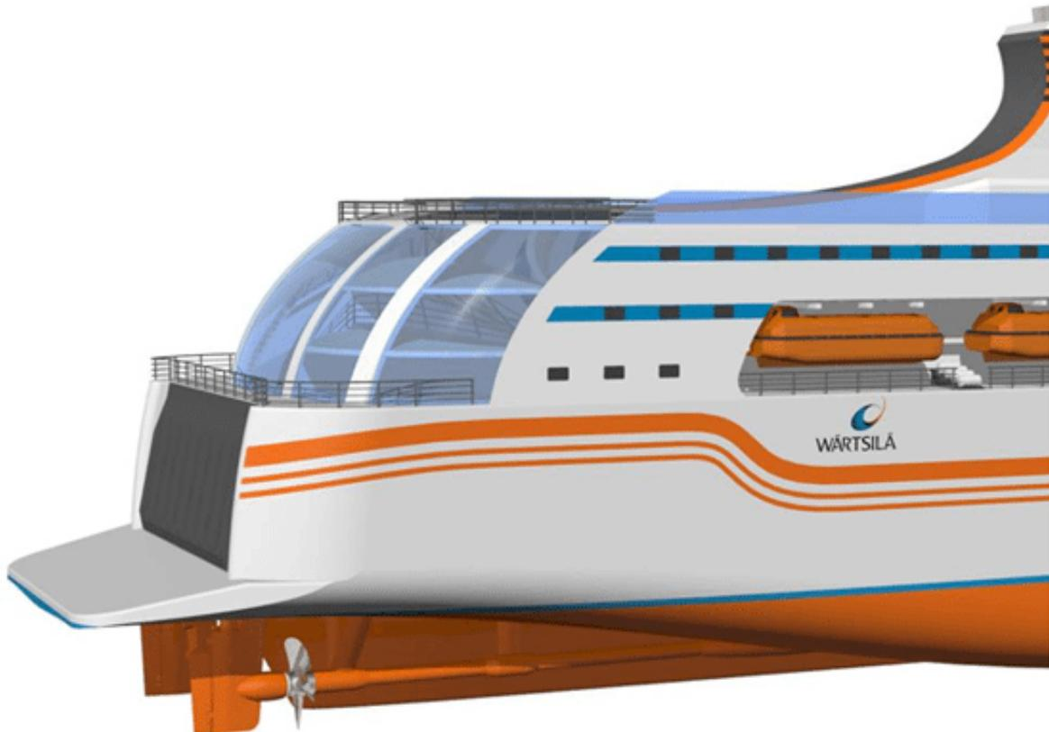
A ducktail is basically a lengthening of the aft ship. It is usually 3-6 meter long. The basic idea is to lengthen the effective waterline and make the wetted transom smaller. This has a positive effect on the resistance of the ship. In some cases the best results are achieved when a ducktail is used together with an interceptor.
