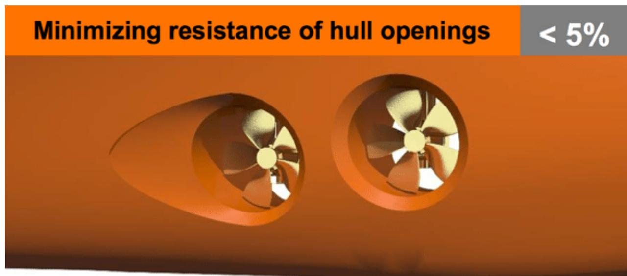
The water flow disturbance from openings to bow thruster tunnels and sea chests can be high. It is therefore beneficial to install a scallop behind each opening. Alternatively a grid that is perpendicular to the local flow direction can be installed. The location of the opening is also important.
