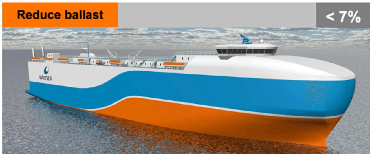
Minimising the use of ballast (and other unnecessary weight) results in lighter displacement and thus lower resistance. The resistance is more or less directly proportional to the displacement of the vessel. However there
